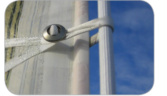
Connection between sail and anti-torsion cable.
